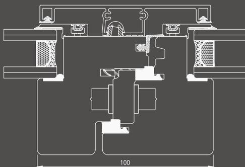
**Central node with profile in aluminium (standard) of Window/French window**
